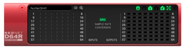
The illustration above shows a RedNet D64R, with a single PSU input and a single, locked network connection, acting as the network master with the Sample Rate Converters enabled.
